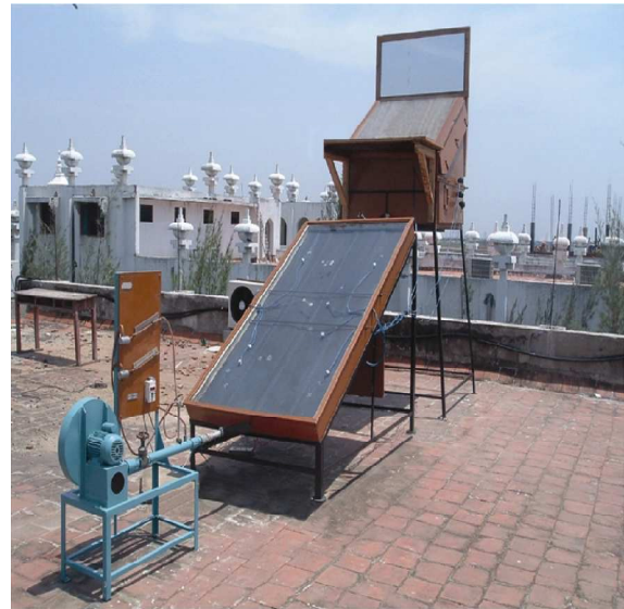
Fig.18. a) Schematic view of the desiccant integrated solar dryer: b) pictorial view of the desiccant integrated solar dryer with reflected mirror developed by V. Shanmugam and E. Natarajan [37, 38].
