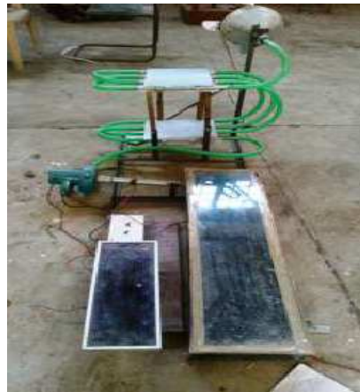
Fig.15. Pictorial view of forced circulation solar dryer system operated with PV cell [22].
