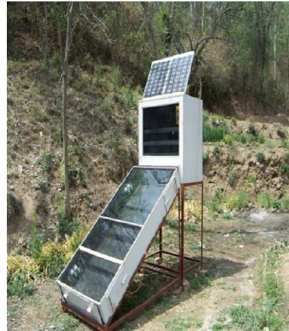
Fig.17. a) Schematic view b) Pictorial view of forced circulation solar dryer for hill products [30].
