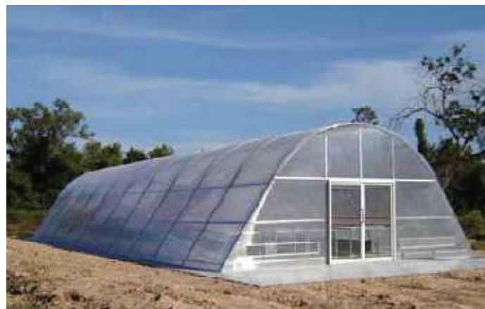
Fig.19 Pictorial view of green house solar dryer used for chilli drying in Thailand [20].
